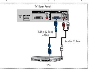
NOTE: The "Anynet" jack is for repairs and software upgrades.
